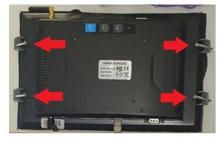
The **VOR-15.6-M-A** is mainly installed in panel mounting mode. This requires cutting a hole in the panel door corresponding to the sizes given in the table above.
