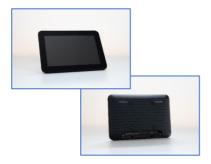
The rear of the screen has 4x fixing points at 75mm centres. Only use the screws supplied otherwise damage can occur to the PCB
